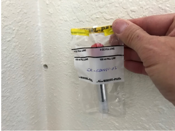
Sample: CVC-CDW01-02 Results: 1.04% Chrysotile IN Joint compound by Point Count Analysis
